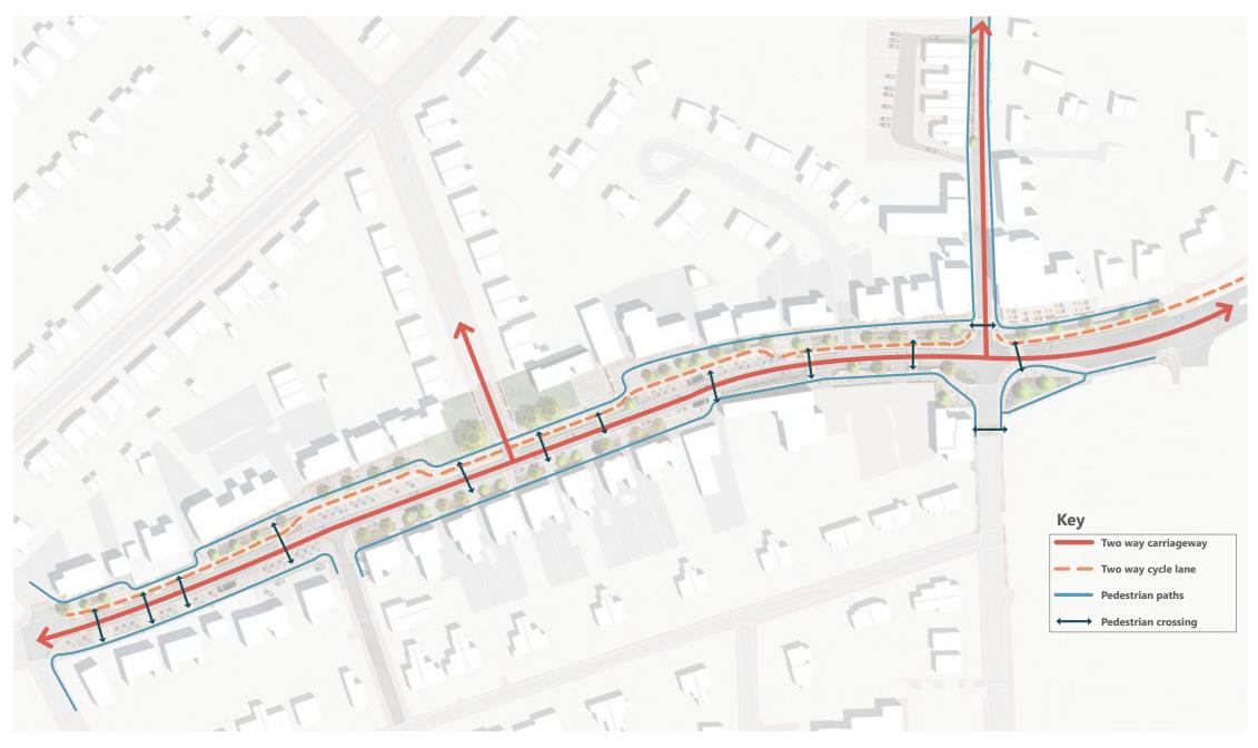
design include changes in texture and colour between different circulation routes, a small lip to edgings that separate circulation routes, tactile paving at crossings and ensuring the appropriate lux levels for street lighting.
