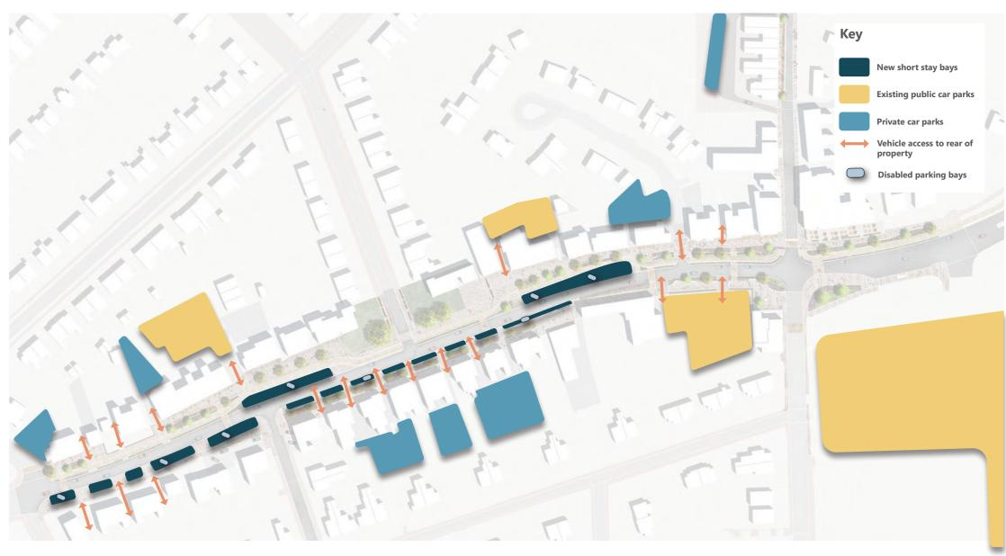
Loading bays and refuge collection points have been positioned at 3 key locations along the road and will avoid the currrent "on road" arrangement that causes congestion and conflict with pedestrians.
